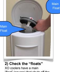
XO coolers have a main "float" (square) that shuts off the water flow when reservoir is full. The cooler **also** has a backup safety float (round) if the first float fails. Sometimes, floats detach in transportation. They need to be attached. Check the floats to make sure they are attached to the Reservoir Lid.
