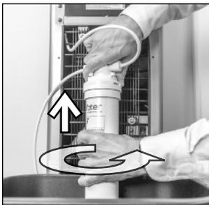
**5. Insert filter into to filter head**
